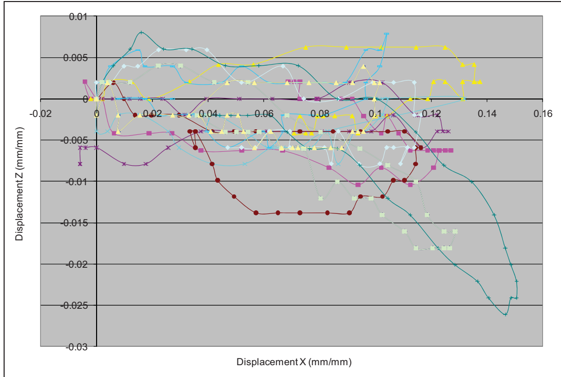
Figure 7-7(a): Trajectory of the cg of the head for 50 th percentile adult male subjects during tensed muscle dynamic impact.
